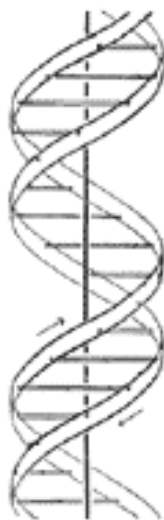
Figure 1. This figure is purely diagrammatic. The two ribbons symbolize the two phosphate-sugar chains, and the horizontal rods the pairs of bases holding the
